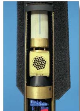
The middle system (M-signal) combines high attenuation of lateral sound incidence, similar to a hypercardioid characteristic (which is about 10 dB), with the large front-to back ratio of the super-cardioid characteristic.
